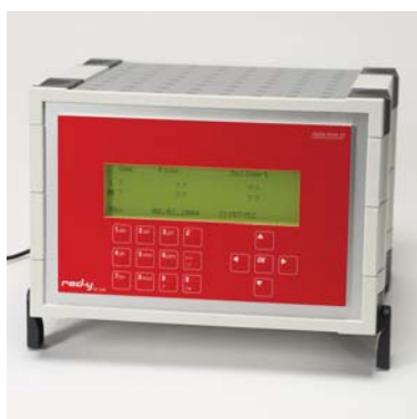
process control unit PCU800
